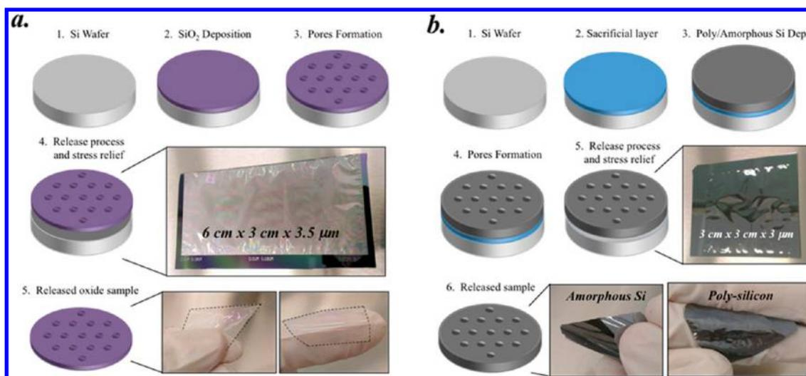
**Figure 1.** Fabrication process flow of silicon dioxide fabric, including digital photographs of a 18 cm<sup>2</sup> silicon dioxide membrane before (step 4) and after (step 5) release from the carrier wafer (a). Fabrication process flow of polycrystalline/amorphous silicon fabric, including digital photographs of 9 cm<sup>2</sup> amorphous and polysilicon fabrics before (step 5) and after (step 6) release from the carrier wafer (b).
